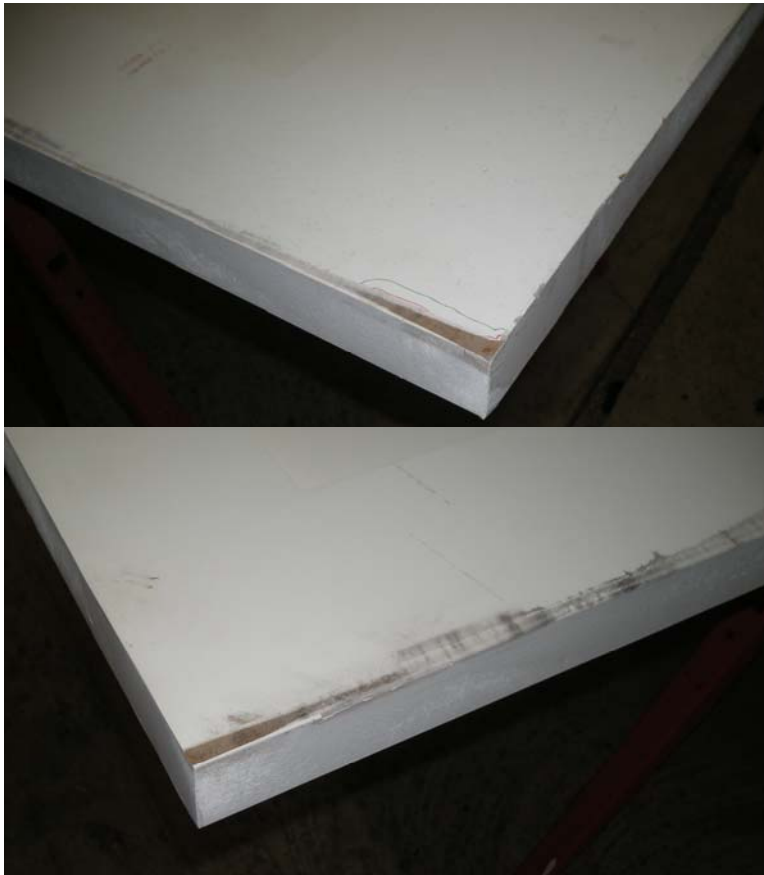
Figure 6.--Paint wear that occurred during the testing.
