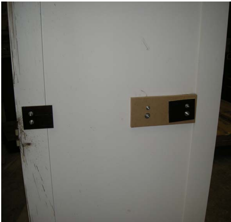
Figure 3.--Pusher bar backer plates.
