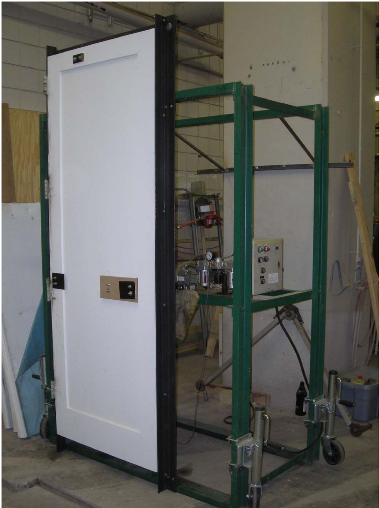
Figure 1.--Cycle slam test fixture with IHS Door attached to frame.
